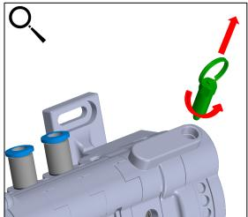
Remove the manual adjustment fixture by unscrewing it by hand.
