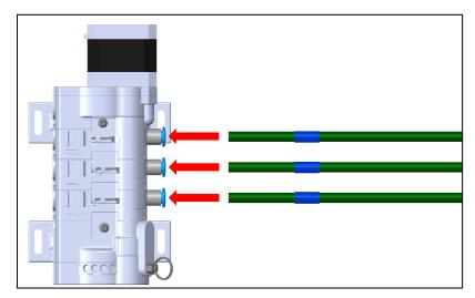
Insert the three long PTFE tubes from the box to the tube connectors of 3Dfeedy.
