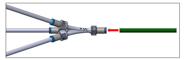
• Insert the short PTFE tube from the box to the tube connector of the PTFE tube collector.
