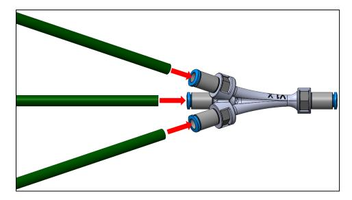
Insert the second end of the three long PTFE tubes to the tube connectors of the PTFE tube collector from the box.
