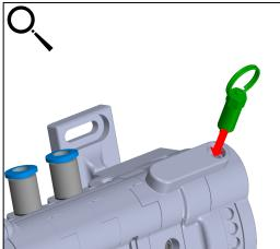
Insert and tighten the manual adjustment fixture hand-tight.
